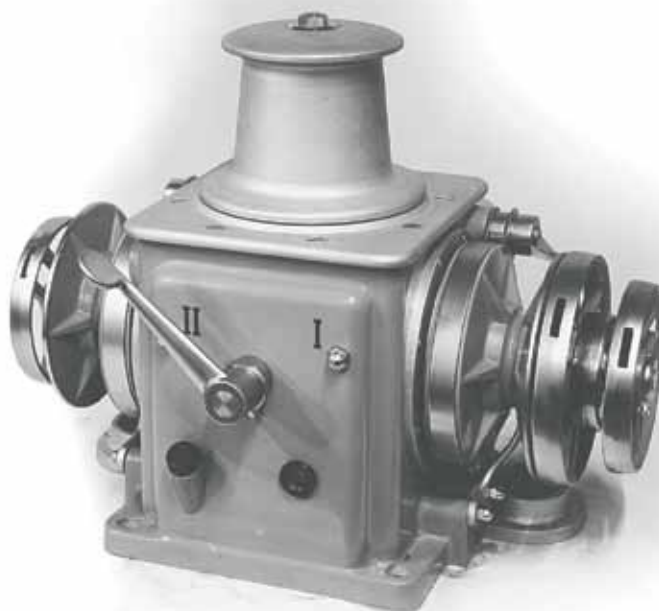
One of first anchor windlasses built in 1966
