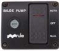
Controls any pump equipped with an automatic float switch. This unit features a black plastic panel. It has a built-in fuse holder and an internally lighted rocker switch with 3 positions (automatic, off, or manual) with the Rule "fail-safe" spring return to "off" from the "manual" position.
