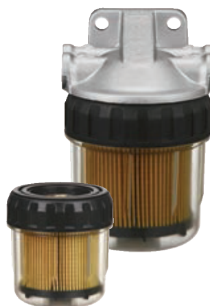
Code 1836-2 FILTER WATER-GASOLINE SEPARATOR WITH REUS- ABLE SEE-THROUGH BOWL KIT Water separator of anodized aluminum. Reusable see-through bowl for 10 Micron filter. Connectors suitable for Mercury/Yamaha outboards.
