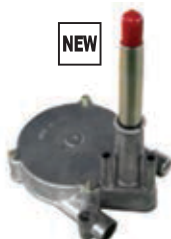
Code 1737-1 HEAVY DUTY STEERING SYSTEM Heavy duty steering system, easy to connect Suitable for boats up to 9 meters and up to 200HP for single engine application. Can be connected with steering cable code 1740 Lock to lock steering wheel turns: approx. 4. Maximum allowable steering wheel diameter : 400 mm. Standard 3/4" tapered shaft of galvanized steel
