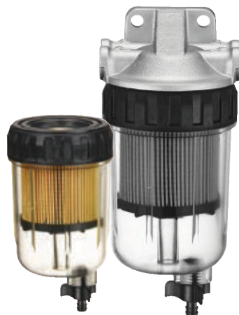
Code 1836-1 FILTER WATER-GASOLINE SEPARATOR WITH REUSABLE SEE-THROUGH BOWL KIT Water separator of anodized aluminum. Reusable see-through bowl for 10 Micron filter. Connectors suitable for Mercury/Yamaha outboards.
