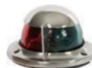
Code 3109 BICOLOR STAINLESS STEEL NAVIGATION LIGHT (Green - red) 112.5° red -112.5° green 12V/10W, Ø 5.5 cm.
